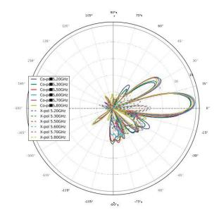
V-POL ELEVATION GAIN (dBi) FOR ZERO AZIMUTH
